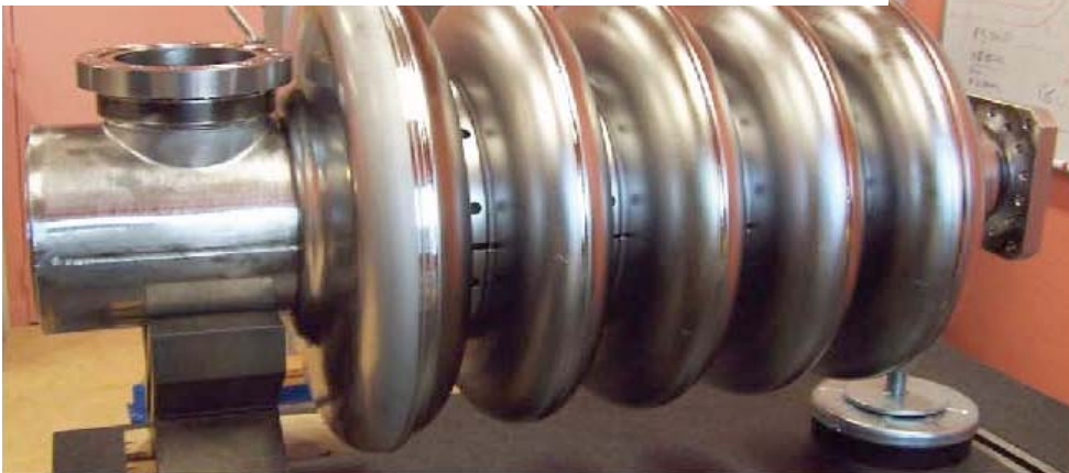
Elliptical 5 cell bulk Niobium cavities (e.g.: \beta=0.47 )
