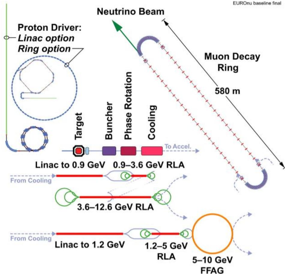
Schematic baseline of the accelerator facility for the neutrino factory.
