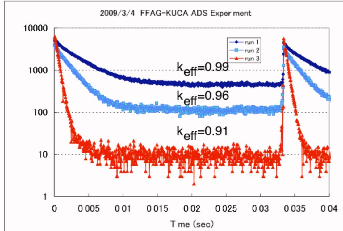
Neutron rate as a function of time for different effective multiplication factors.
