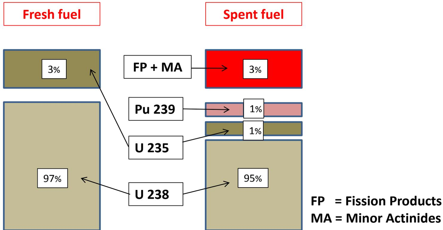
⇒ Highly inefficient use of the fuel resources in critical Light Water Reactors.
