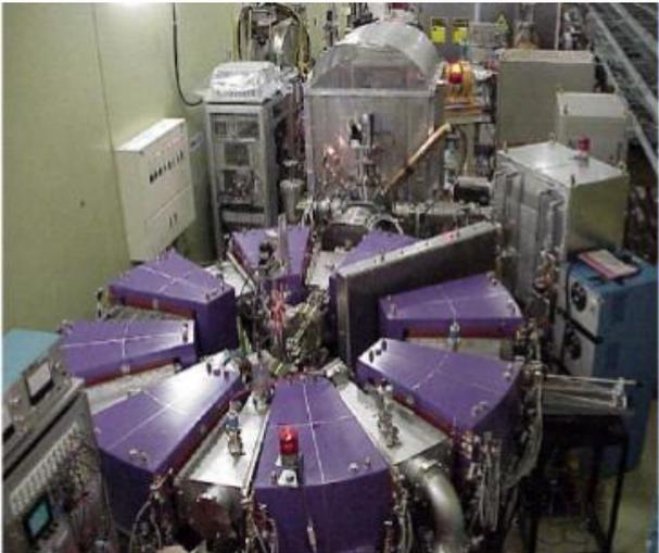
PoP machine 500 keV machine, 2.5 m diameter, operated in 1999 in KeK.
