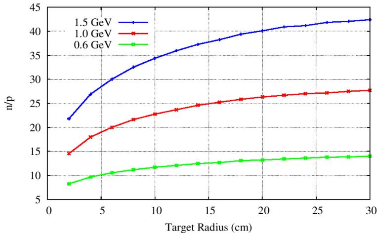
Target multiplicity on a cylindrical lead target.
