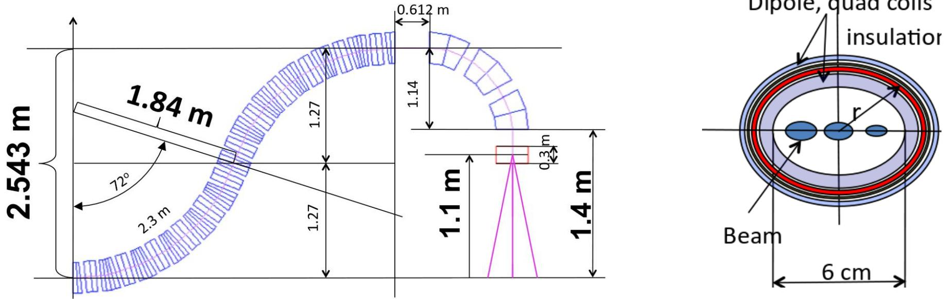
FFAG magnets sequentially arranged along the beam tube of the gantry.
