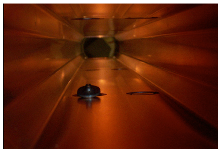
Fig. 20. A button of an upper BPM fell off onto a lower button (left plot). Melted feed-through of a lower button and the fallen upper button (right plot).
