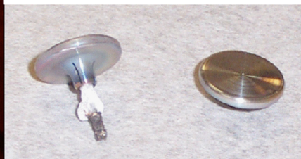
Fig. 20. A button of an upper BPM fell off onto a lower button (left plot). Melted feed-through of a lower button and the fallen upper button (right plot).
