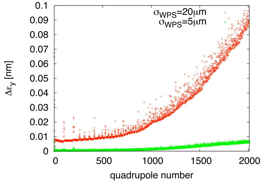
$\Rightarrow$  Significant impact of wire position sensor accuracy
