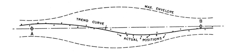
→ To simulate the « absolute » uncertainty of position of the CLIC components along the linac, using the Survey standard tools, in order to get additional input for the simulations of the beam dynamics.
