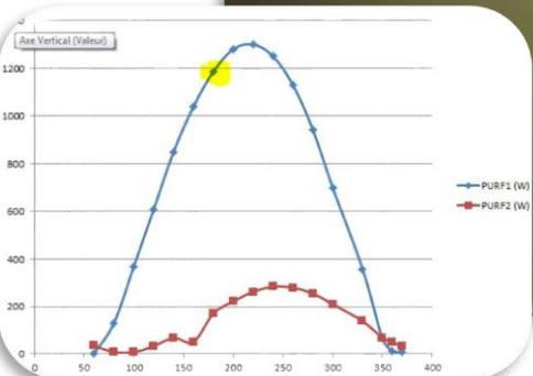
We had arcing in the air side when reaching 1 MW full reflection with few SW phases
