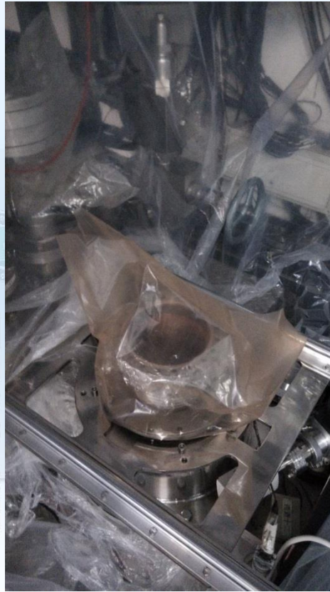
The coupler port covered with clean PVC plate (down) and plastic film (up)
