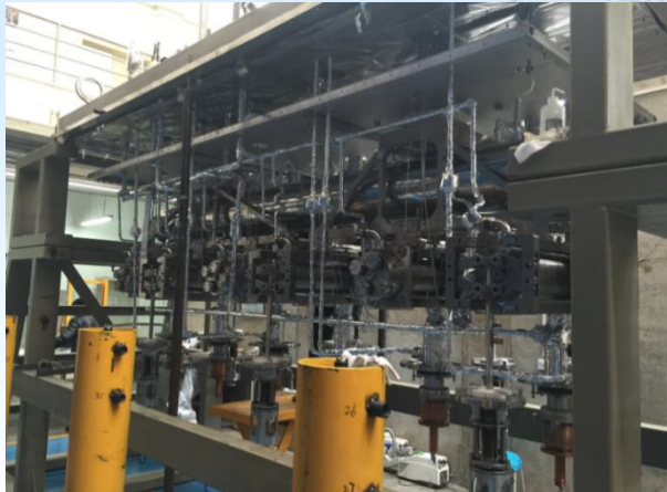
CM1 of Injector-II for C-ADS: cuboid shape cryo-module
