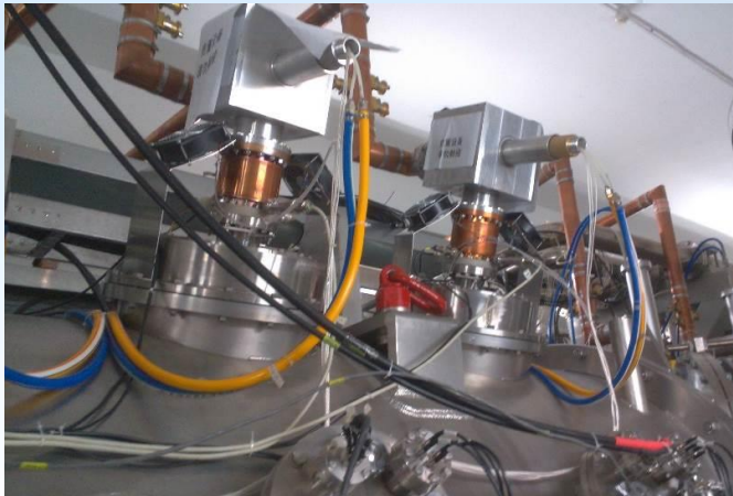
FPCs assembled with CM1 of Injector-I
