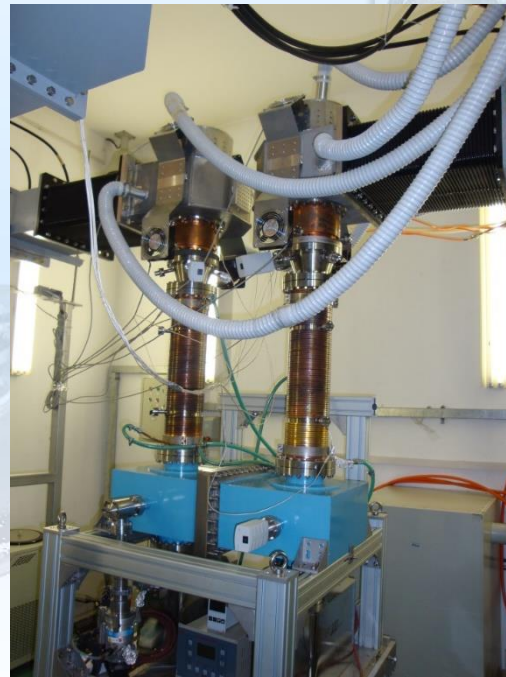
High power test stand for 500MHz FPCs
