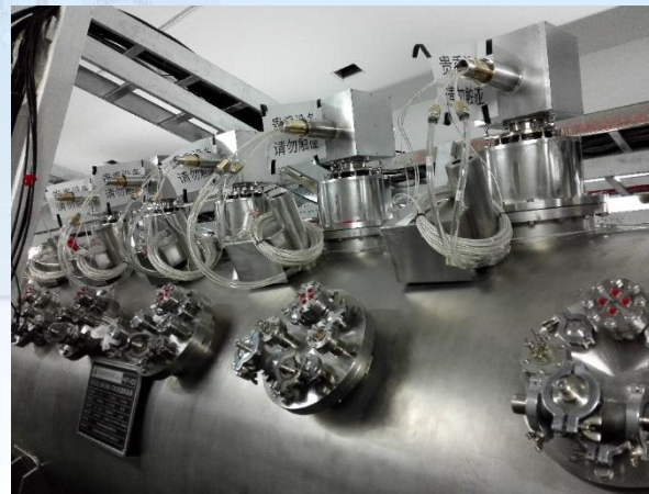
FPCs assembled with CM2 of Injector-I
