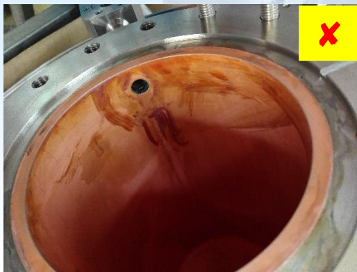
Bad coating: blemishes and oxidation
