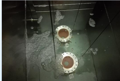
Outer conductor ultrasonic clean
