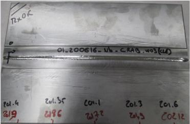
Average shrinkage measured (Retraite soudage):**0.6mm**
