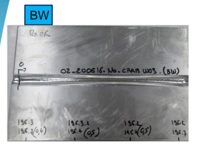
Average shrinkage measured (Retraite soudage):**0.5mm**
