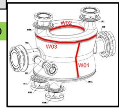
Average shrinkage measured (Retraite soudage):**0.45mm**
