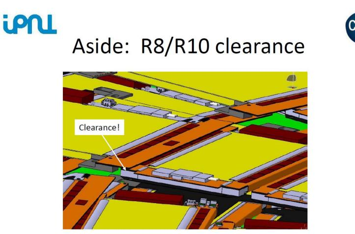
The fact that the PS and 2S modules are now staggered in Z gives clearance (0.6mm) between the PS frontend chips on R8 and the underside of the 2S hybrid on R10 This clearance should be increased (to 1.0mm) by adjusting the height of the cooling inserts *or by raising the 2S hybrid with respect to the sensor*
