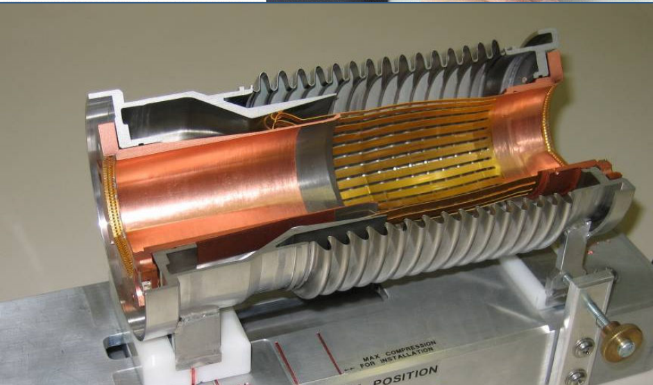
Arc plug-in module at working temperature
