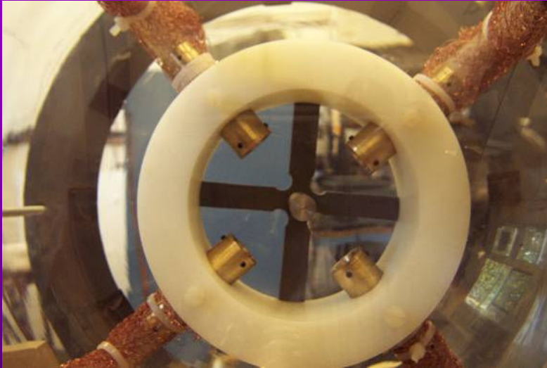
POS (mock-up) with 4 plasma guns and central cathode
