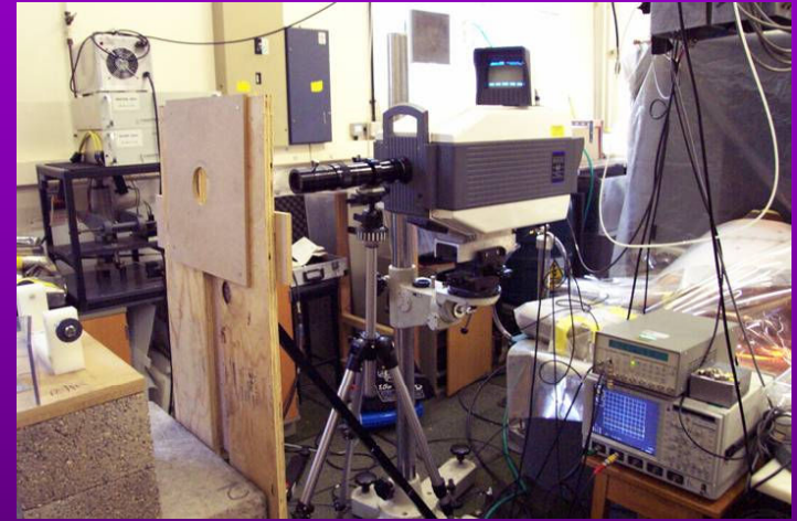
Imacon 468 (John Hadland) Nikon lens, 8 frames 10 ns gating speed
