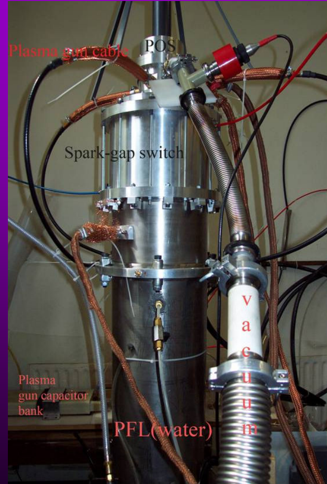
POS installed on top of generator
