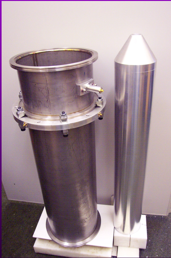
Pulse forming line 3.8 \Omega / 53 ns
