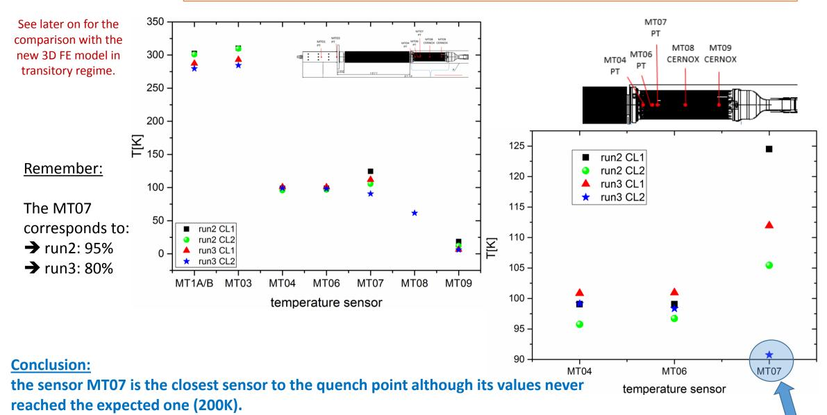
The highest temperature value detected by MT07 sensor is 124.5K for run2 in CL1.
