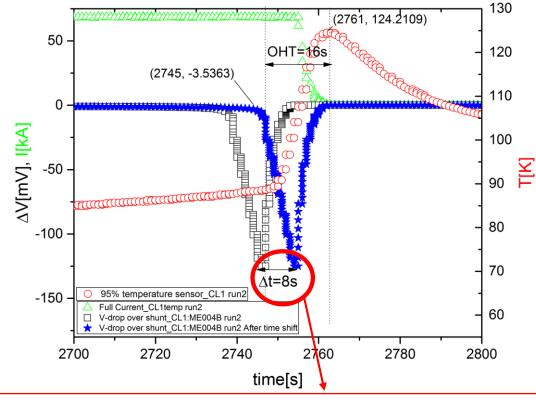
${\bf N.B.}$  time shift of 8s due to the two acquisition systems: QDS for V and CODAC for T and I
