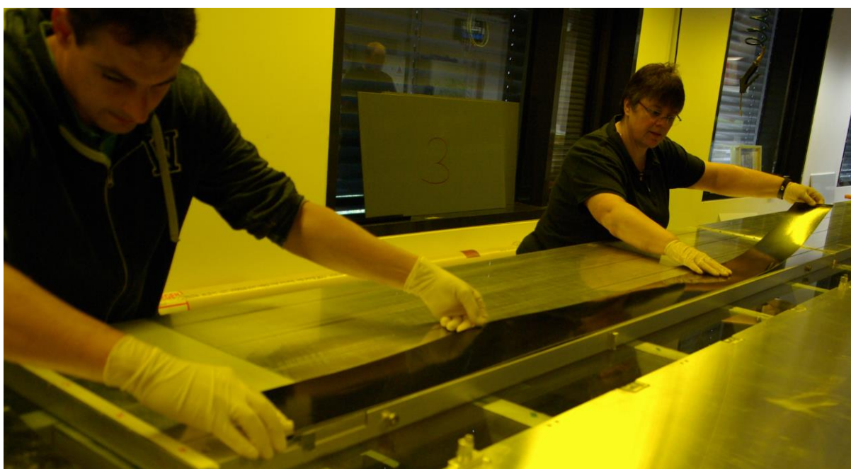
Figure 37 Placing mats to the gluing jig
