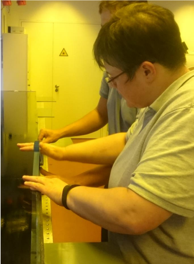
Figure 64 PET-tape to avoid the glue spreading out
