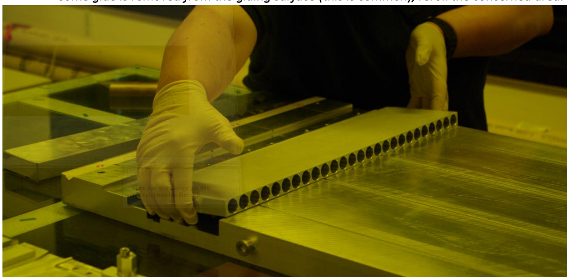
Figure 35 Endplug in gluing jig
