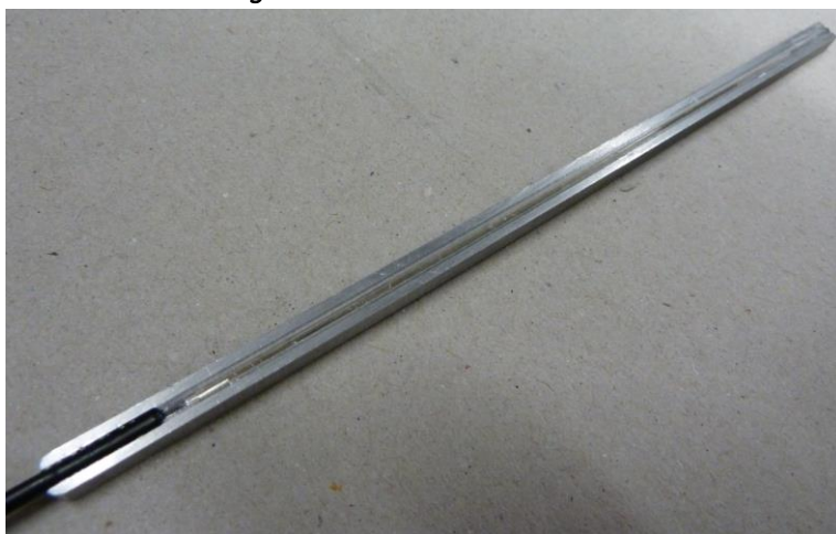
Figure 14 Cured light bar with fibre
