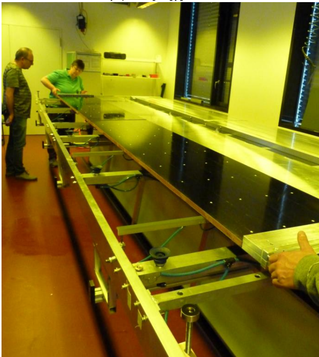
Figure 58 Half module been pushed on the gluing jig
