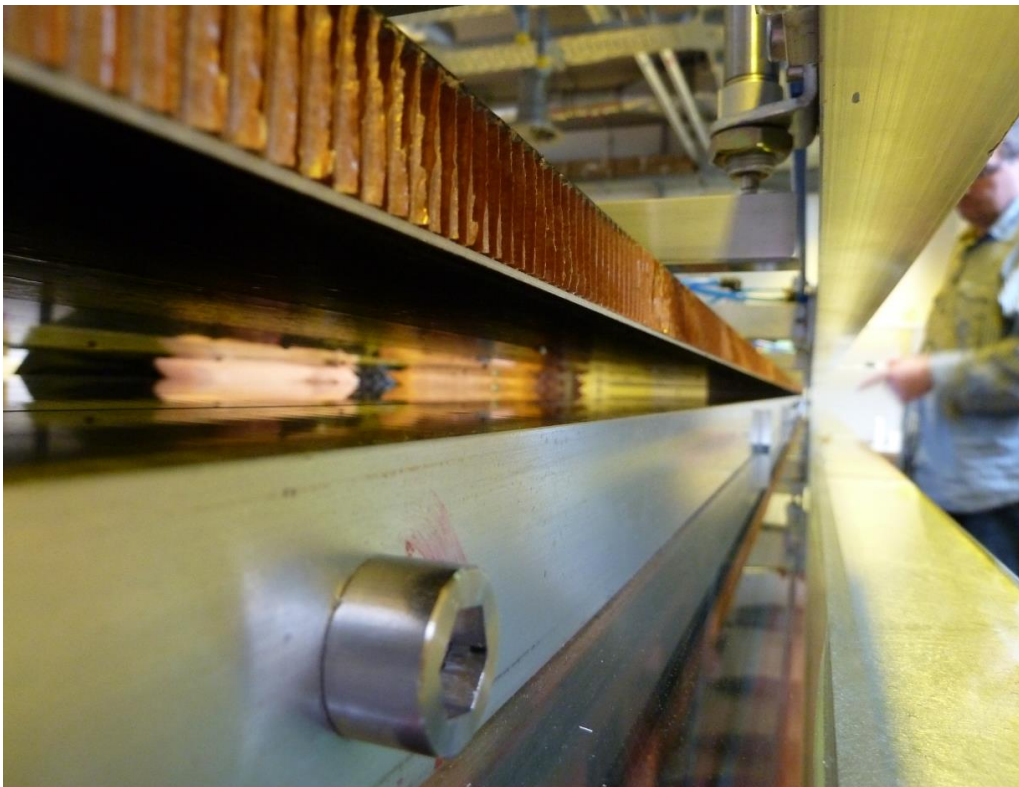
Figure 52 Mats lifted from gluing jig
