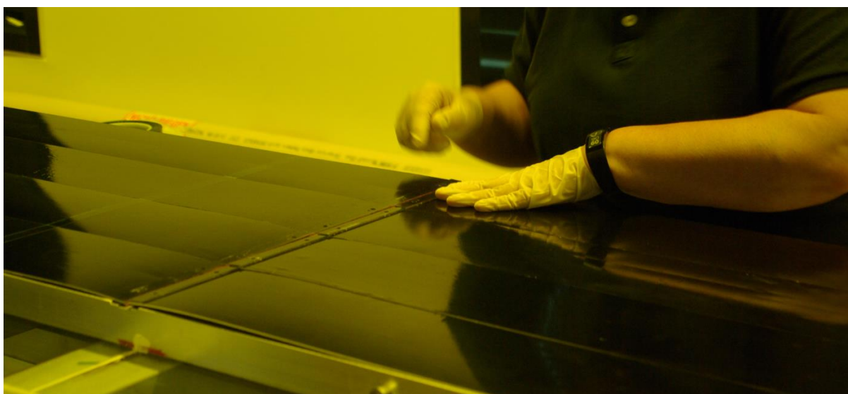
Figure 37 Placing mats to the gluing jig
