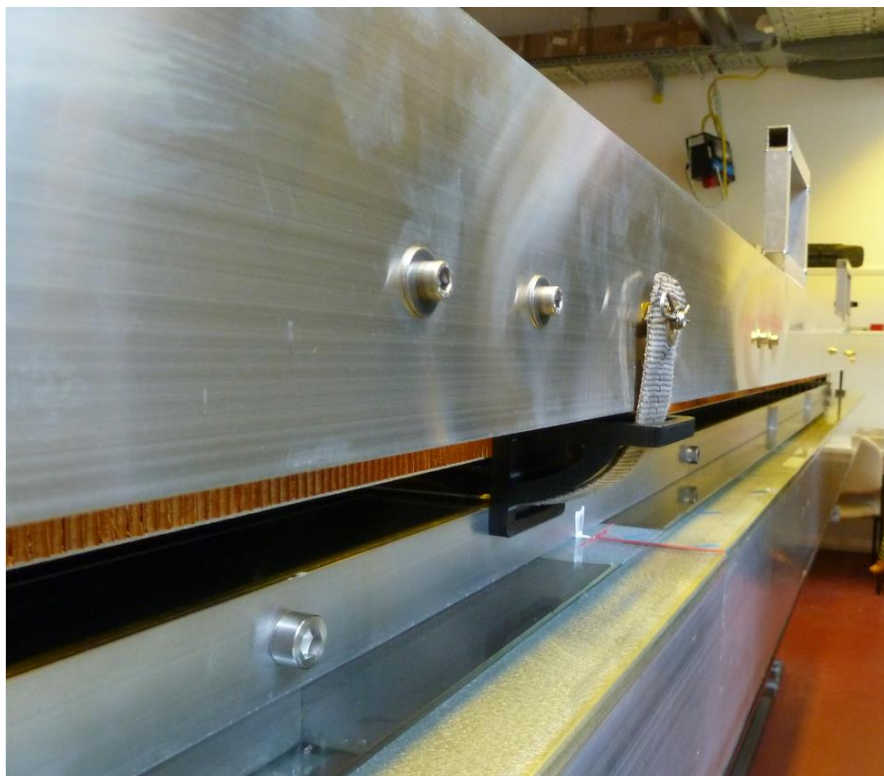
Figure 54 “Security belt” attached to the “Lifting and Turning device”.
