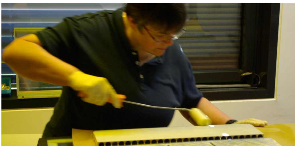
Figure 33 Applying glue with the roller to the endplug
