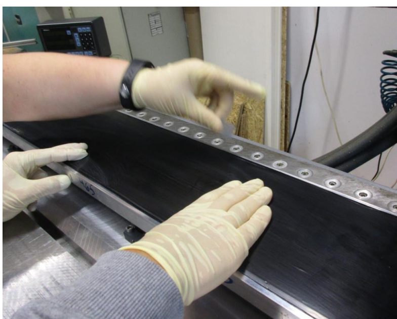
Figure 26 Insuring pins of mat going into the alignment groove in the jig
