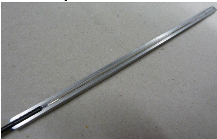
Figure 14 Cured light bar with fibre
