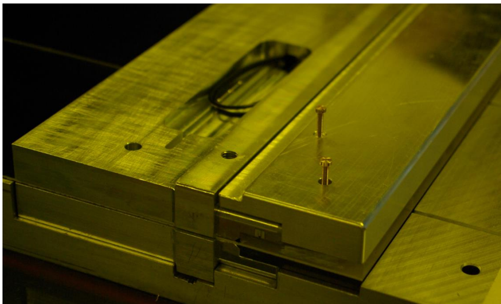
Figure 43 Insure proper fitting of the dowel pins into the endplugs and endpieces
