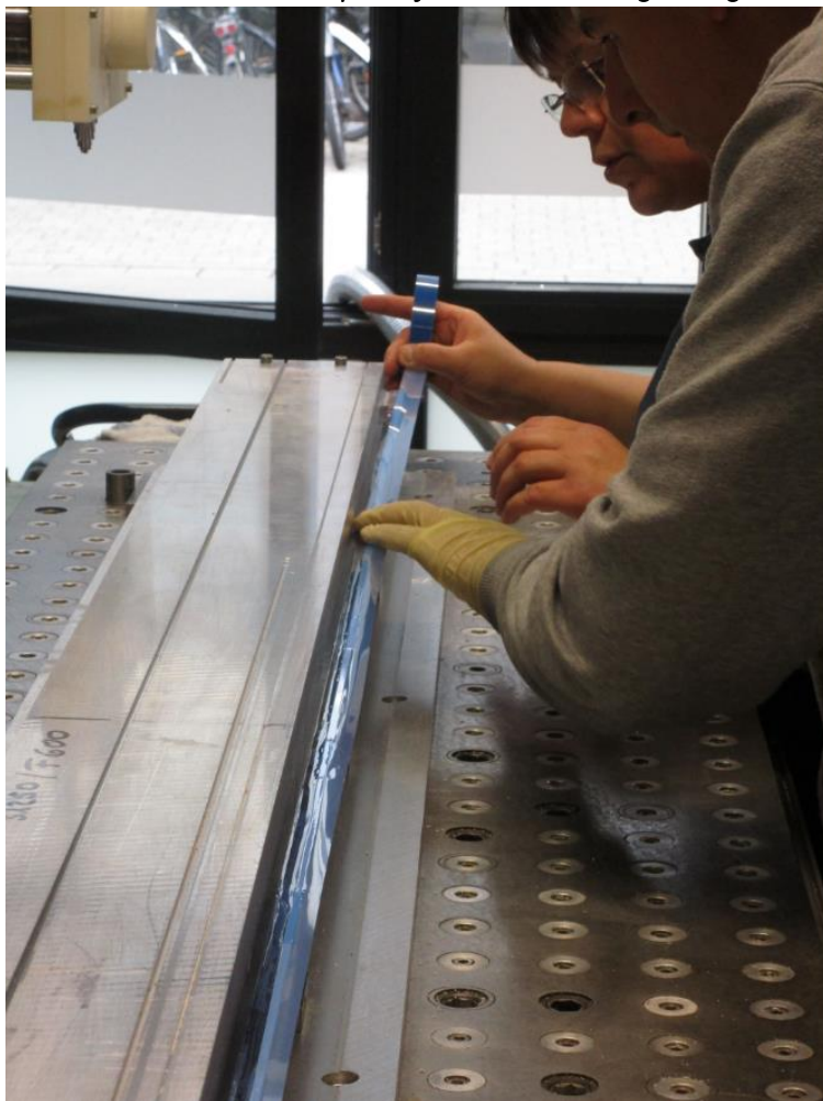
Figure 28 Tape on cut sides of the mats
