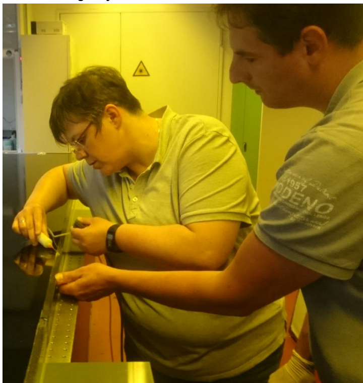
Figure 63 Applying glue between side walls and polyimide surface of panels
