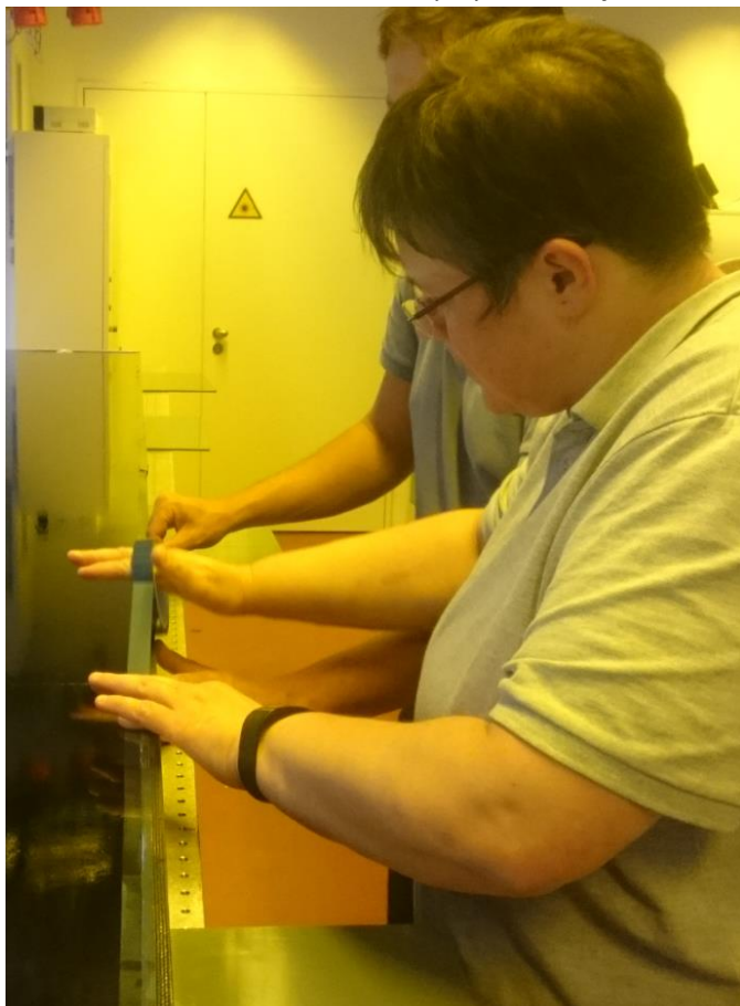
Figure 64 PET-tape to avoid the glue spreading out
