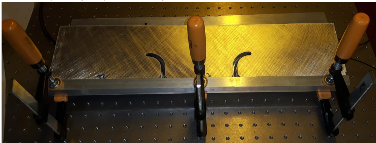
Figure 23 Fastening clamps on Al-bar (the Teflon spacers are not shown on this picture)
