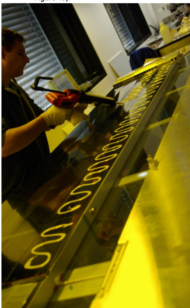
Figure 44 Applying the glue with the glue applicator in sinuous lines
