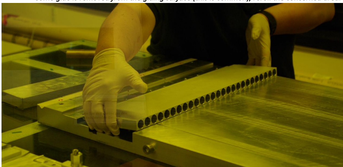
Figure 35 Endplug in gluing jig
