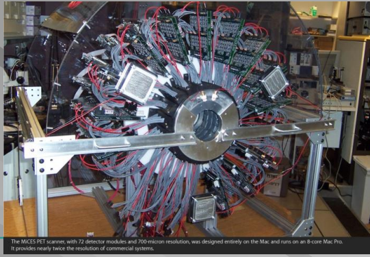
The MICE PET scanner, with 72 detector modules and 200-micron resolution, was designed entirely on the Mac and runs on an 8-core Mac Pro. It provides nearly twice the resolution of commercial systems.
