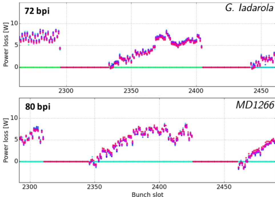
Trains of 80 bunches should allow for  $\approx 2800$  collisions in IP1&5 ( $\approx +2\%$  in lumi)
