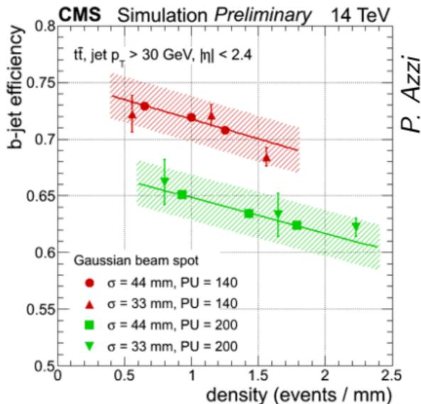
Pile-up density deteriorates relevant *signals* in a linear fashion → **Effective density is the average**
