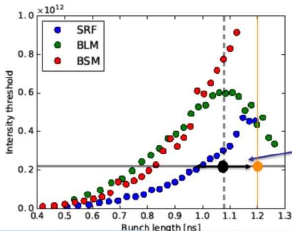
Need 10% margin taking into account bunch length variation bunch-to-bunch with **single RF** (no need for 800 MHz system)
