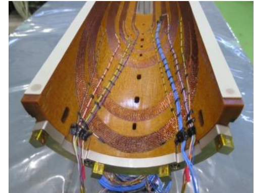
Strain gauges to monitor axial preload
