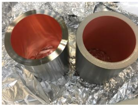
Cu-SS sputtering for FPC outer conductor
