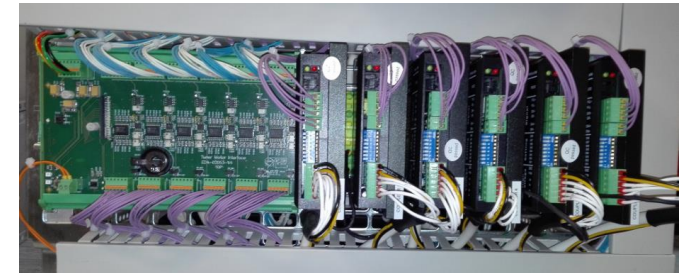
An example of 6 motor controller for HIE-Isolde tuning system
