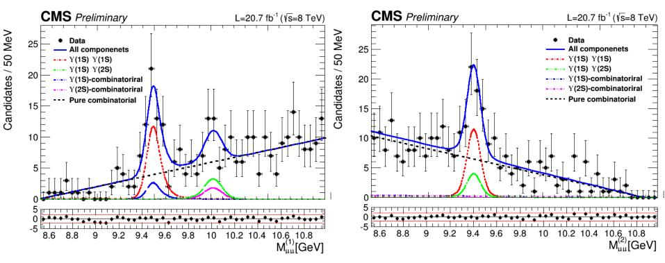
Main selections: Yield extraction from maximizing 2D likelihood PDF --signal is modeled by two Crystal-ball functions --background is modeled as 1<sup>st</sup> order polynomial
