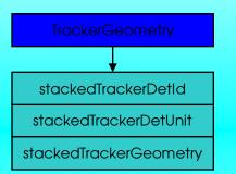
StackedTrackerDetUnit: An object containing a sorted list of the DetIds of the stack members and having a StackedTrackerDetId.
