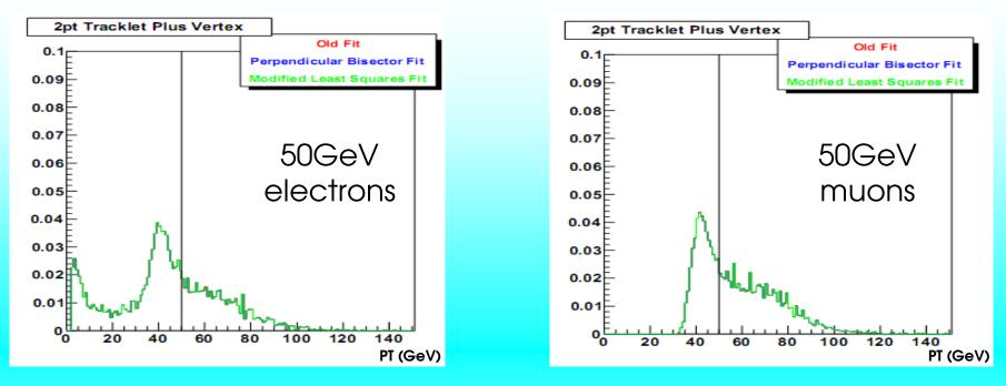
Resolution is poor due to close spacing of layers (using more tracker points improves this)
