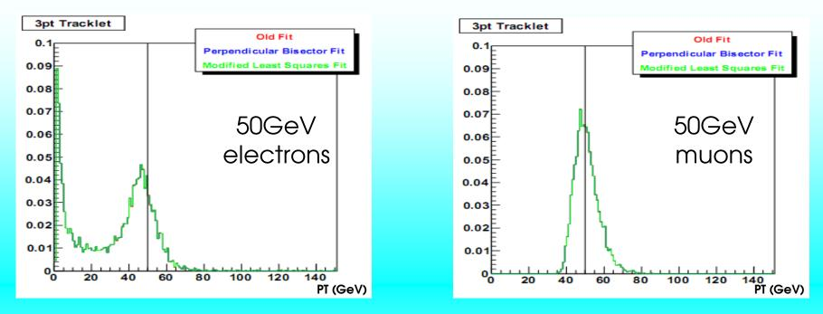
Using three points in the tracker improves muon momentum resolution
