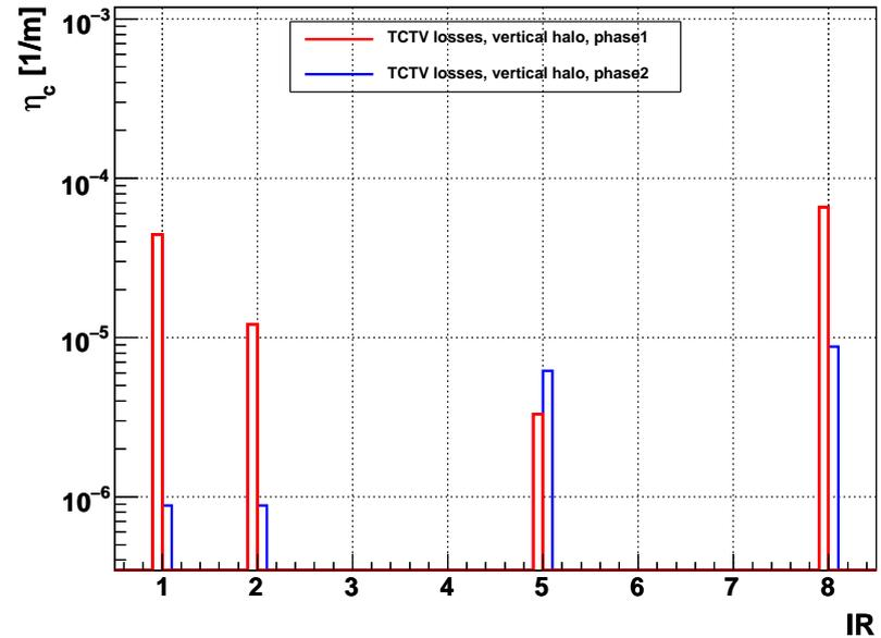
The proposed upgrade solution also reduces load on the tertiary collimators (background) in front of the experimental insertions. No change in losses on tertiary collimators in IR5 due to missing cryogenic collimators in dispersion suppressor in IR3.
