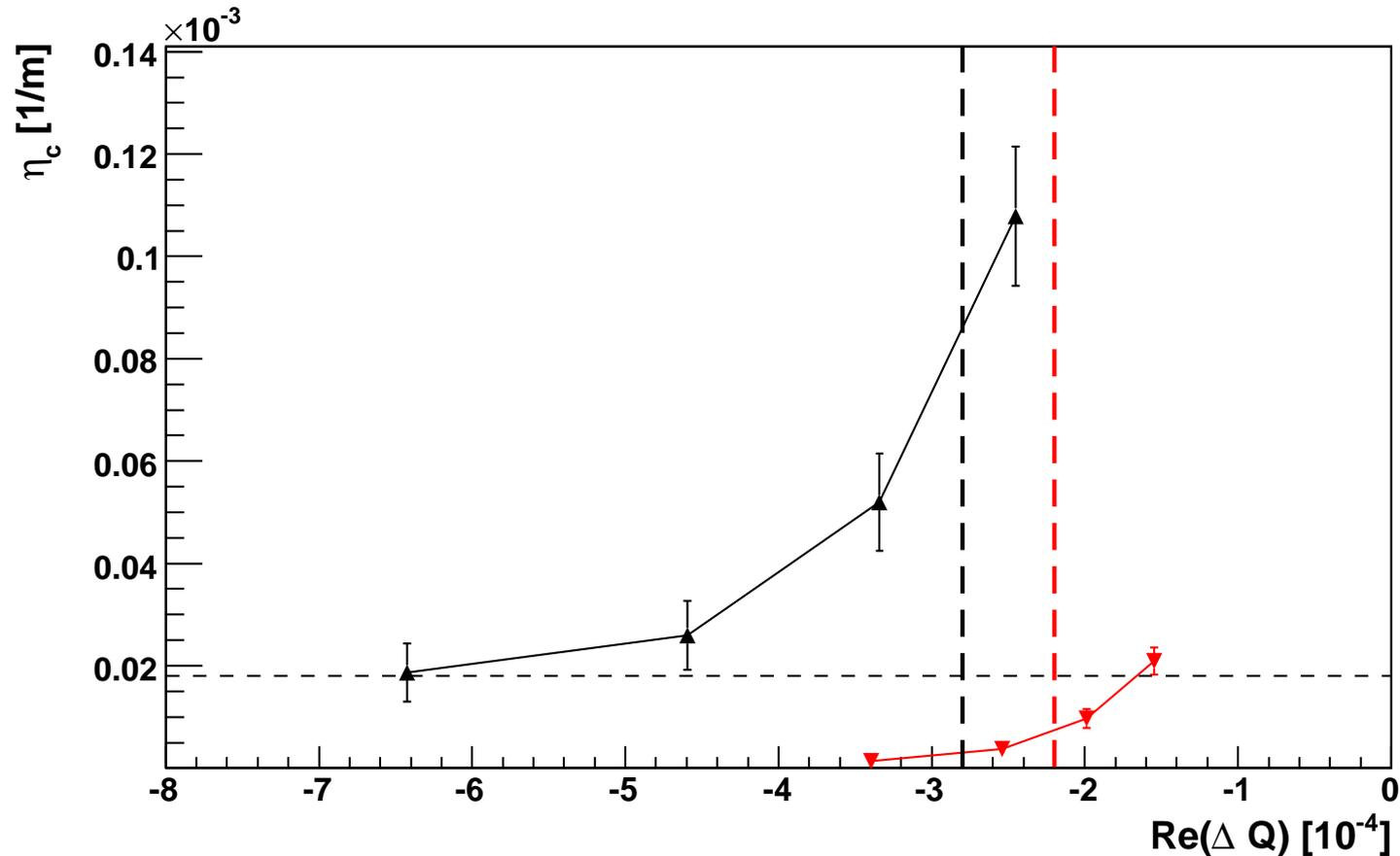
Only for phase 2 with cryogenic collimators one finds settings to stay below the required  $\eta_c$  and within the stable region.
