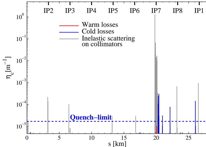
Loss map including jaw flatness error, collimation setup errors (tilt, offset and gap-size) and machine alignment errors.
