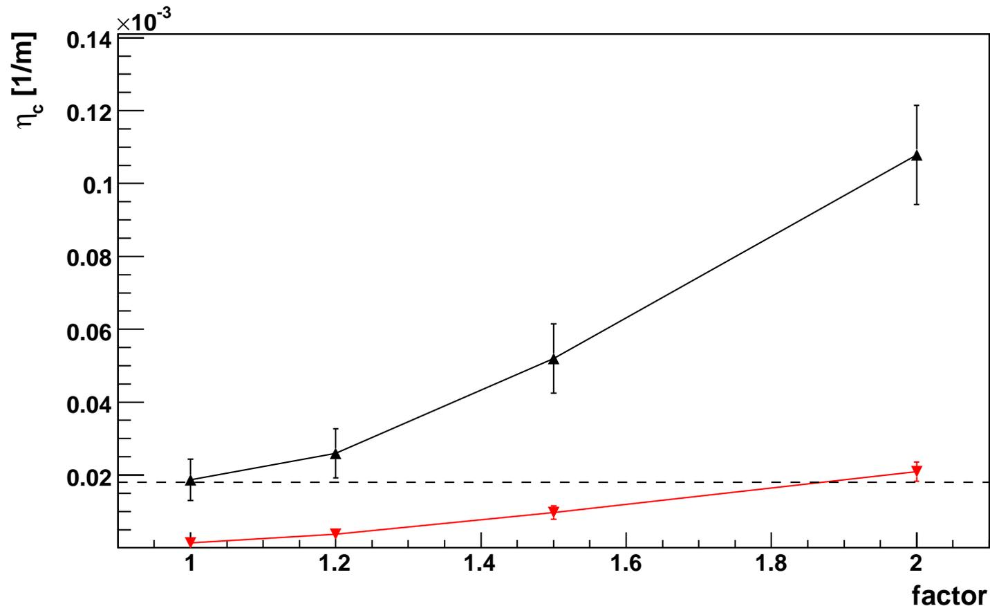
**Reminder:** multiplication “factor” is only true for TCP and TCS collimators. For **phase 2** and ideal machine, opening the gaps up-to a “factor” 1.5 possible.  $\Rightarrow$  increased triplet aperture needed or  $\beta^*$  has to be adapted.
