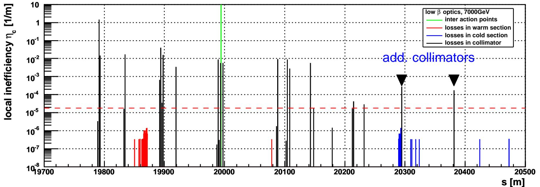
Copper secondaries set to nominal settings, carbon secondaries set to relaxed opening ( $26.5\sigma$ ), cryogenic collimators (material copper, length 1 m) placed at 298.89 m and 388.44 m from IR7 at  $15\sigma$ .
