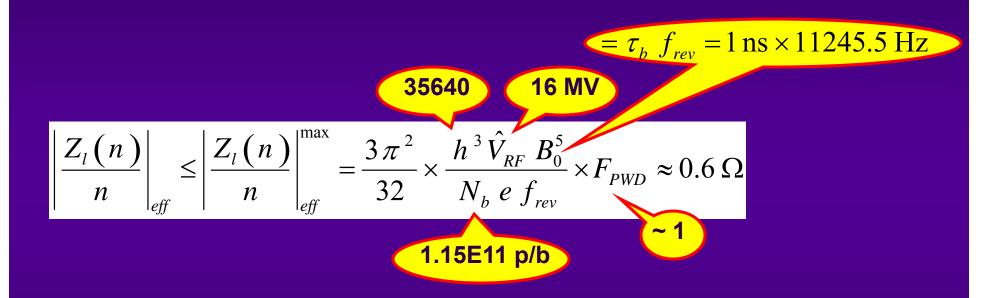
Reminder: In the LHC Design Report (Vol. 1, chap. 5) the effective Broad-Band impedance was estimated to  $\sim 0.1~\Omega$  for the squeezed optics  $\Longrightarrow$  If the imaginary part of the longitudinal impedance is increased (too much) then one could be limited by this mechanism. To be followed-up with Elena Chapochnikova
