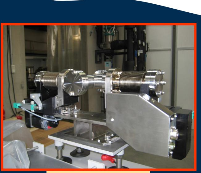
DC Current Transformer (DCCT) Measures the electron beam intensity using a principle similar to the one of FCT. Additionally, a second magnetic modulator detects the beam DC component.
