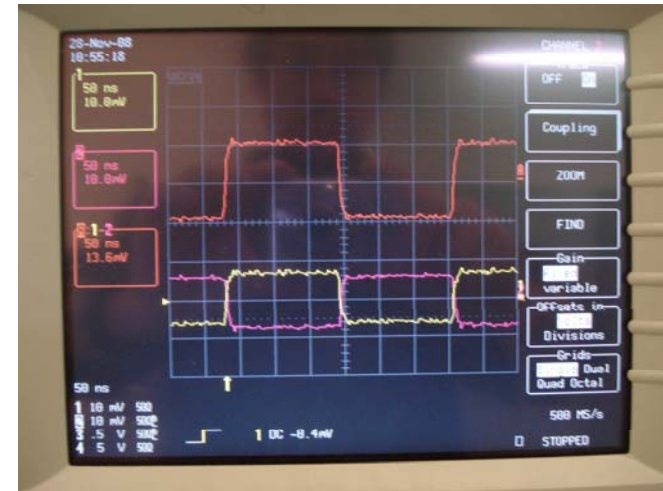
Sigma signal, Calibration AFE bypass (so, the calibration signal don't goes inside the amplifier box)
