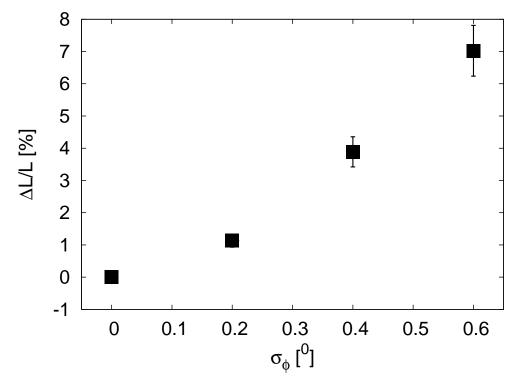
Example of simulation results, a perfect machine is used with a coherent drive beam phase jitter
