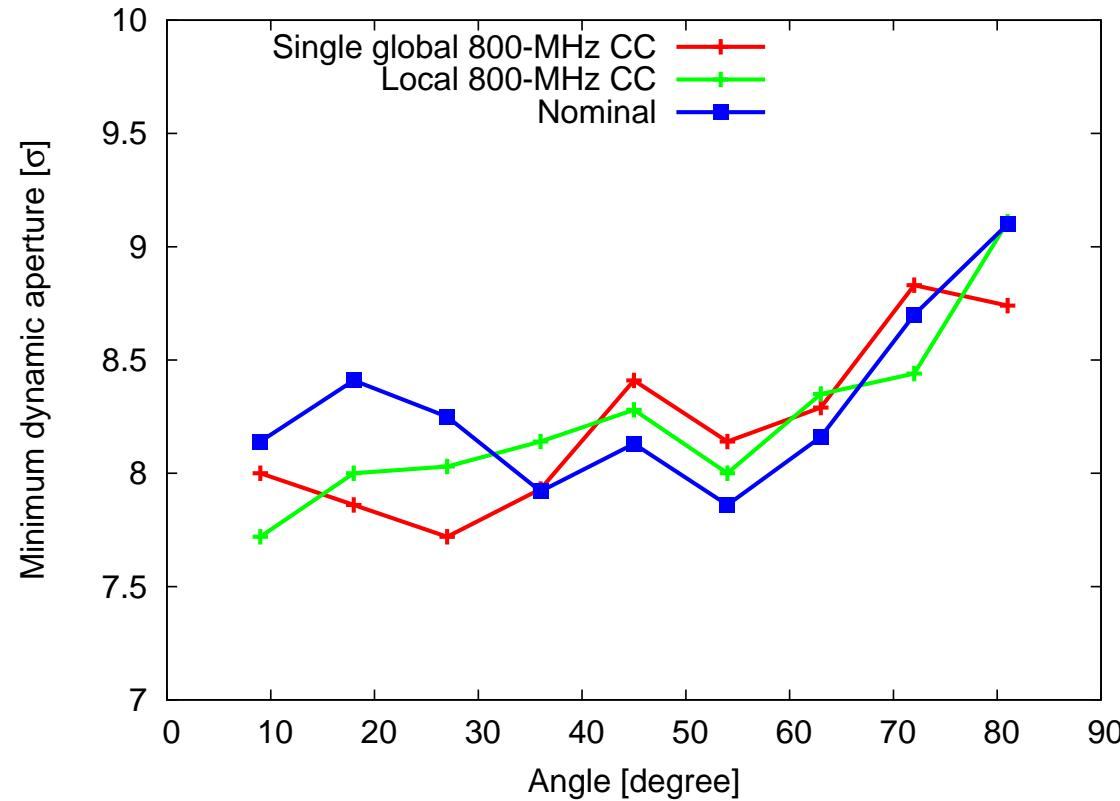
Minimum dynamic aperture over 60 error seeds for nominal LHC optics with or without crab cavity; with all the head-on and long-range beam-beam interactions at IP1, IP2, IP5 and IP8. The dynamic aperture tracking is performed for **100,000 turns**.
