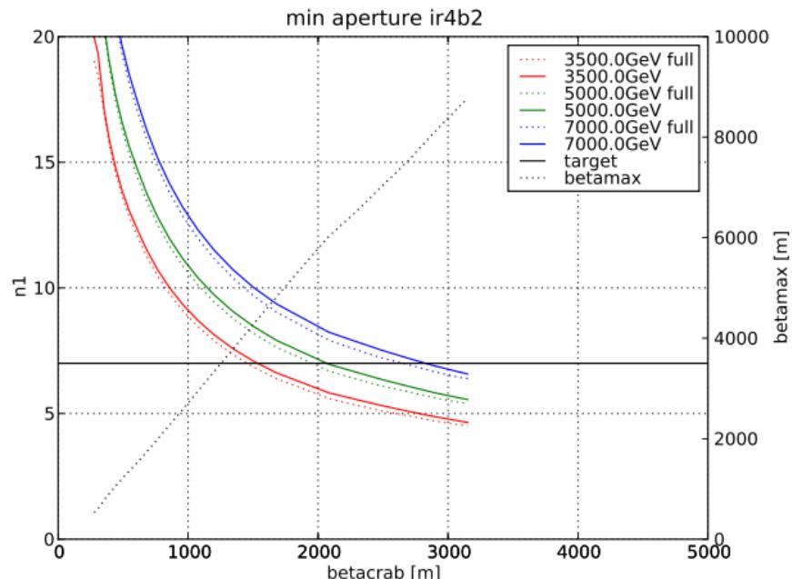
As the emittance decreases with energy, each step of the squeeze has a minimum energy that is compatible with the aperture. This information allow to choose betacrab and energy depending on the purpose of the test and machine conditions.
