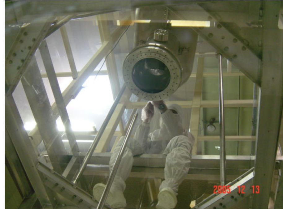
High Pressure Water Rinsing by 80 bar Ultra-Pure water
