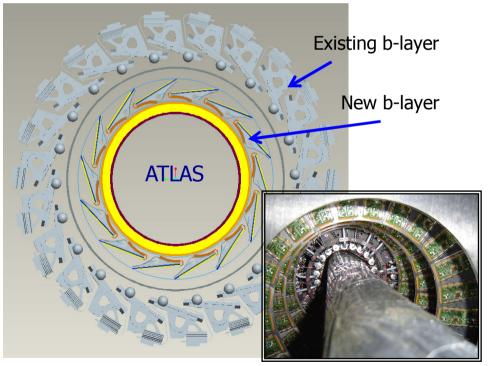
Add new b-layer around a smaller beam pipe, stave structure, 160 MHz readout,  $CO_2$  cooling
