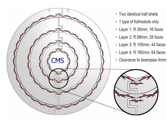
Full substitution : 4 barrel layers + 3 disks per side, weight a fact 3 down, 160 MHz readout,  $CO_2$  cooling
