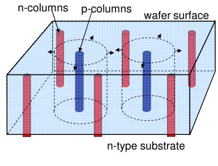
3D silicon : 250  $\mu m$  have been tested , high eff.  $\sim~10^{16}$  p,n/cm², S/N  $\sim~60$
