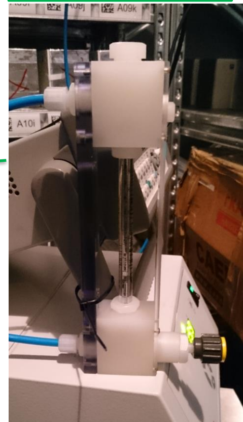
gas flow meter
