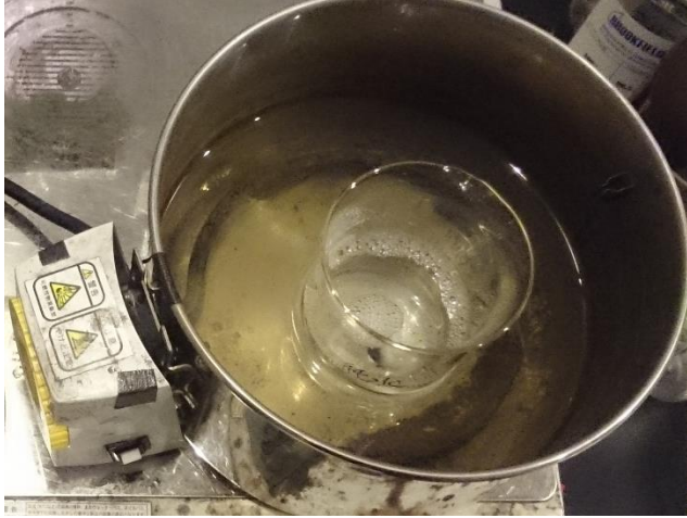
Thermostatic bath; ~ 35deg. (Gelatin in beaker)
