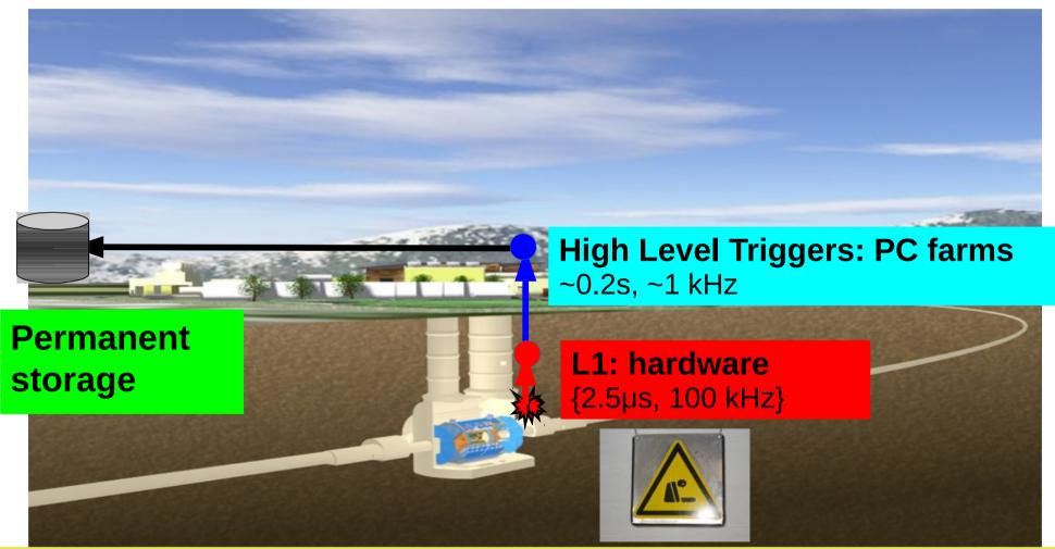
Trigger & DAQ : Select events and get the data from the detector to the computing center for the first processing.
