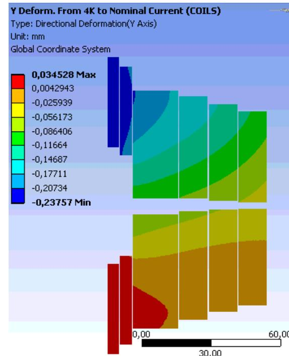
*Coils RELATIVE displacement in mm:
