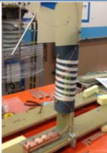
Assembly of 1st 2-layer REBCO CCT
