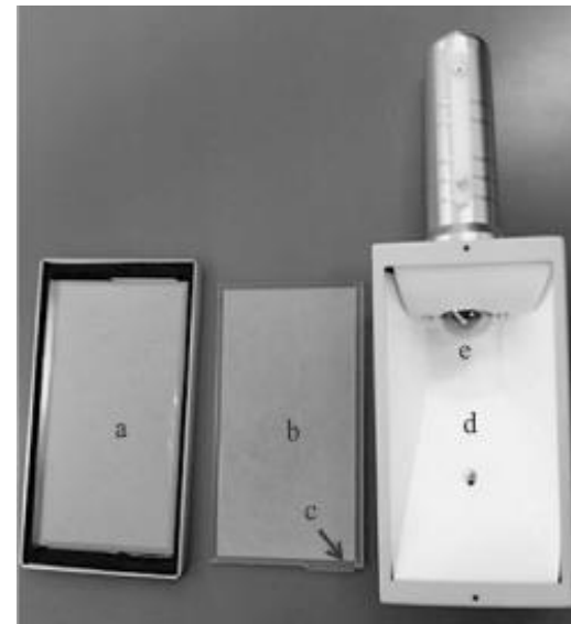
Fig. 1 The inside of a survey meter. From the left, a) light-shielding curtain of thin aluminum foil, b) PEN sheet, c) acrylic sheet support, d) reflection section of white celluloid, and e) photomultiplier tube.
