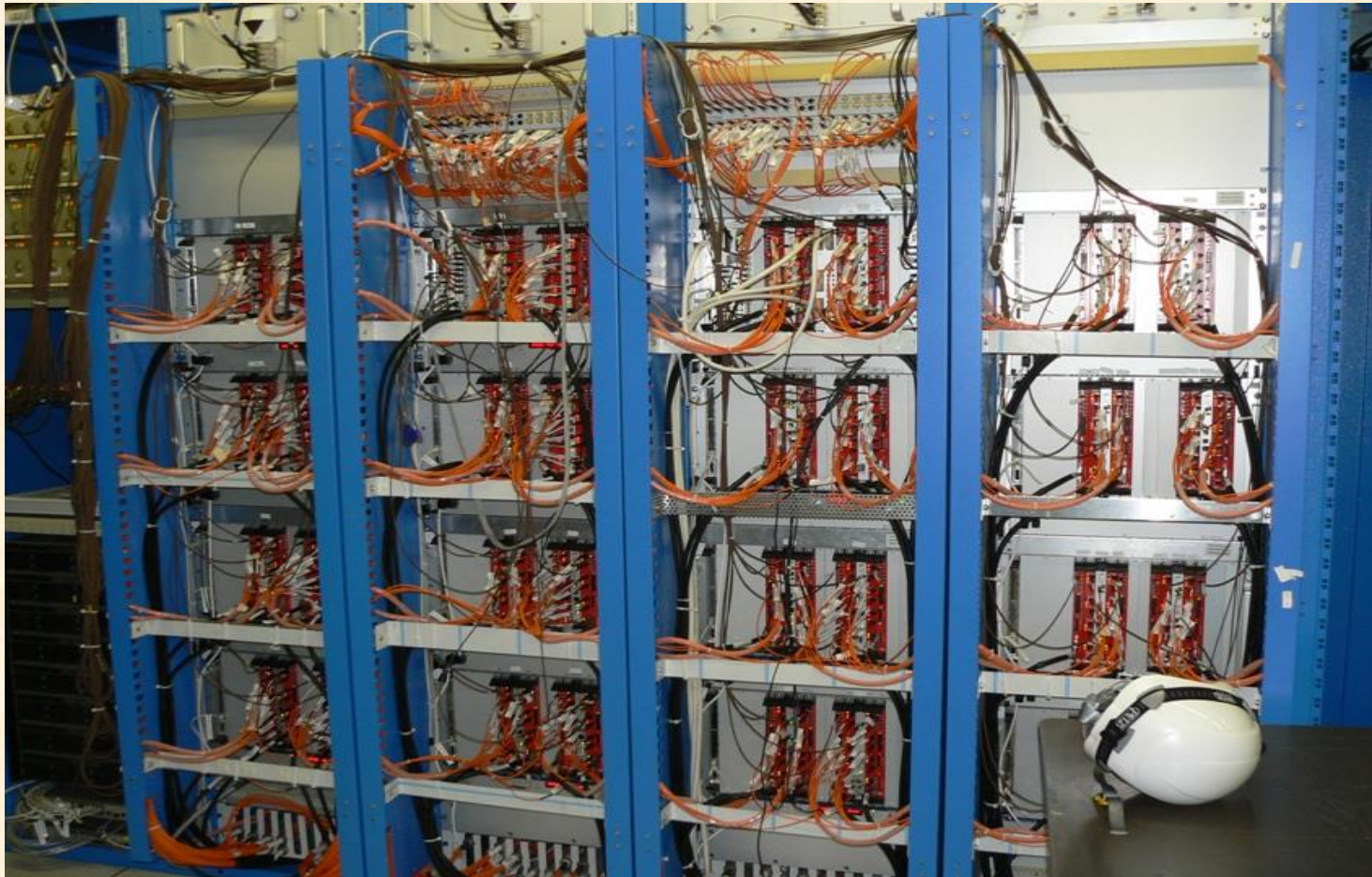
The VMEbus crates of the ATLAS RPC detector
