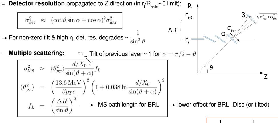
→ Combination of BRL+Disc structure in tilted geometry decreases MS effect:  $\sim \frac{1}{\sin^3 \vartheta} \rightarrow < \frac{1}{\sin^2 \vartheta}$
