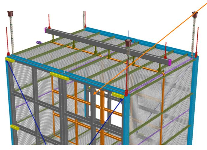
**Anode Plane Assemblies:** 4.1 x 2.5 m wire plane frames (4) tiled to create two drift regions
