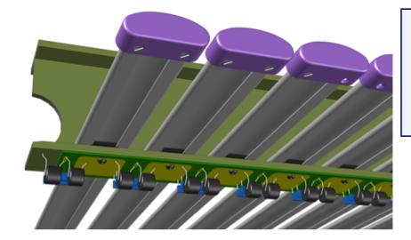
**Field Cage:** roll-formed metal profiles installed in panels (16). Some are removable for detector access. Similar to protoDUNE-SP design.
