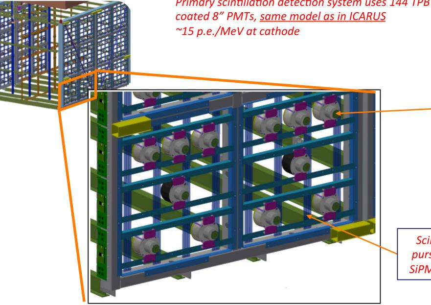
Primary scintillation detection system uses 144 TPB
