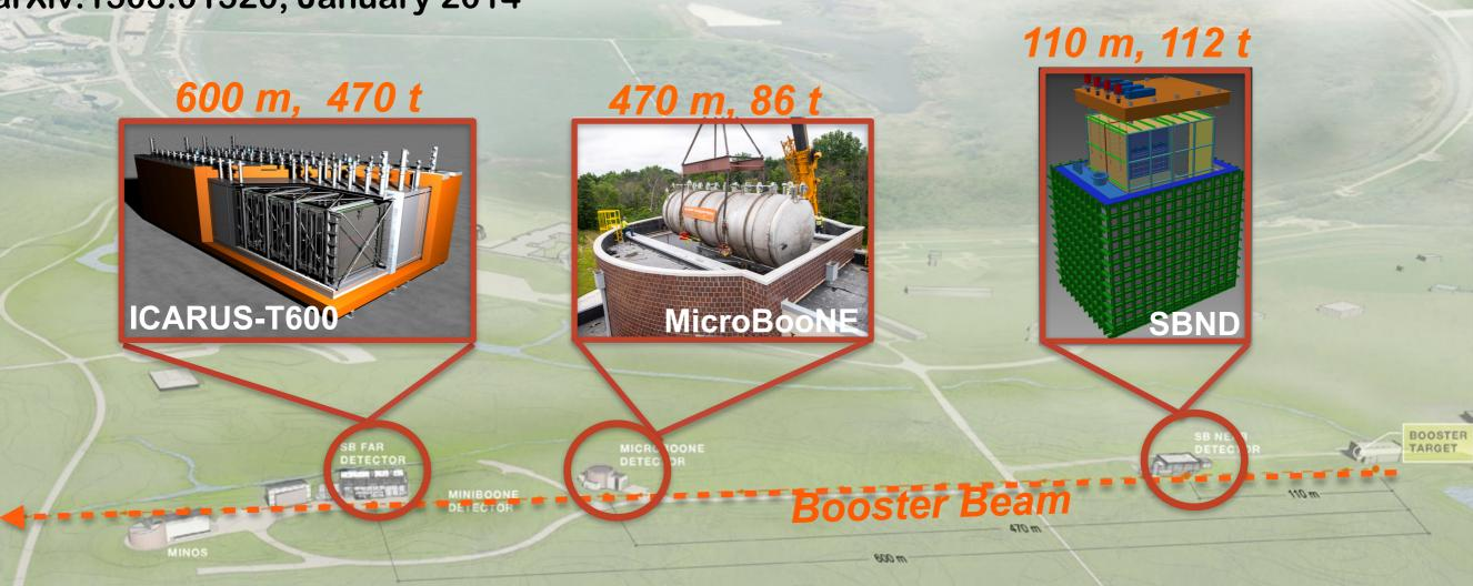
**SBN program - Phase 2 -** By 2018, the MicroBooNE detector will be joined by two additional LAr-TPC detectors at different baselines
