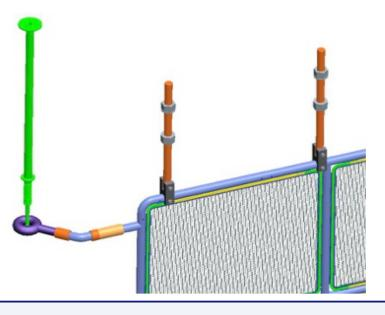
HV & Cathode: SS tubing frames with mesh panels
