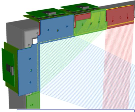
Front-end electronics with cold ADC and multiplexing 11k channels → 4 feed-throughs (MicroBooNE, 8.2k→11 feed-throughs)
