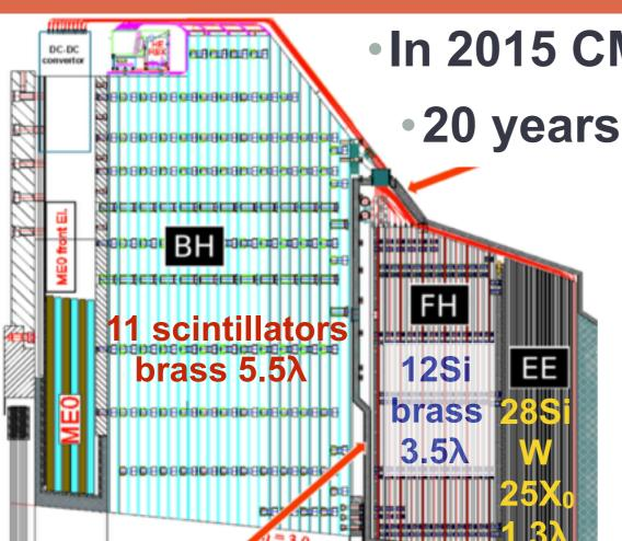
In 2015 CMS chose a silicon based calorimeter
