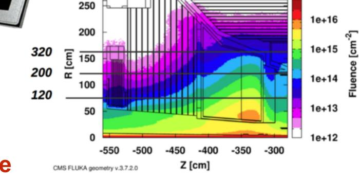
1MeV neutron equivalent in Silicon, HGC, 3000fb<sup>-1</sup>
