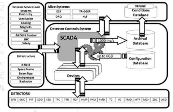
In the LHC, a Detector Control System is a hardware and software component that measures and controls millions of parameters concerning the environment variables.
