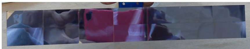
14 ALPIDE chips connected to flexible PCB
