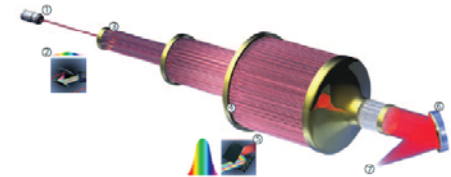
Figure 1 | Principle of a coherent amplifier network. An initial pulse from a seed laser (1) is stretched (2), and split into many fibre channels (3). Each channel is amplified in several stages, with the final stages producing pulses of ~1 mJ at a high repetition rate (4). All the channels are combined coherently, compressed (5) and focused (6) to produce a pulse with an energy of >10 J at a repetition rate of ~10 kHz (7).
