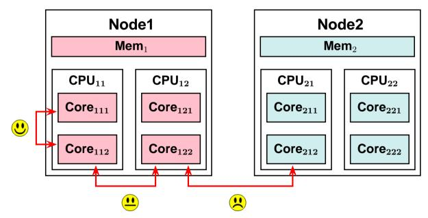
1 process runs on 1 core but too much processes on one node can cause lack of memory.
