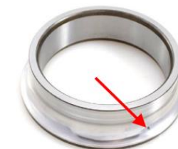
Fig. 2: The inner ring with 2 flaked areas. One flaked area is identified by the arrow.
