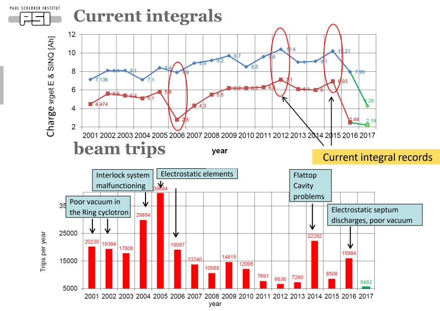
Trips due to discharges at the septum's reach from 300 trips/week to 2000 trips/week (after) breaking the vacuum, or while damaged by the beam). Beam trips have an impact on the availability. To power up the machine again takes about 60s. Only 50 beam trips per day means <u>2% lost availability</u>!
