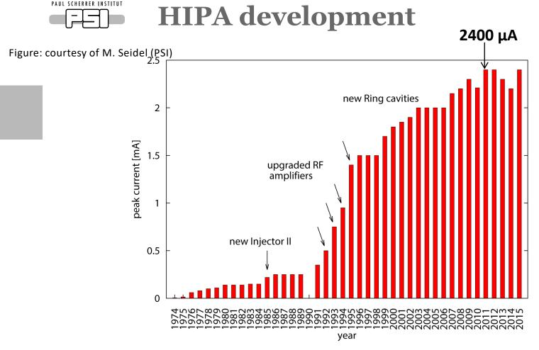
$\circ~$  Beam current increased from 100  $\mu A$  (1974) to 2400  $\mu A$  @ 590 MeV (stable test operations 2015)
