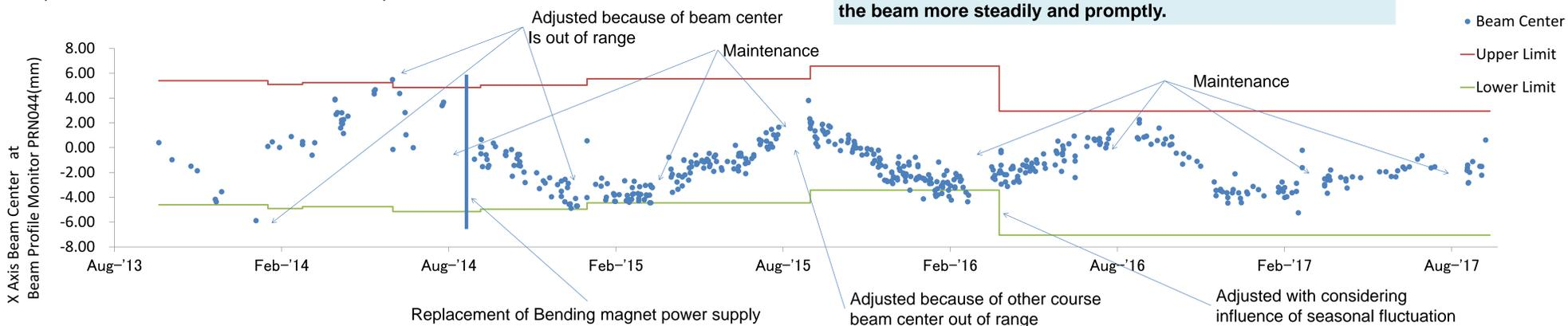
Fig 5 Fluctuation of C350MeV/u beam center at beam profile monitor PRN44
