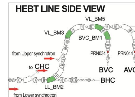
Fig 8 Side view of high energy beam transport line
