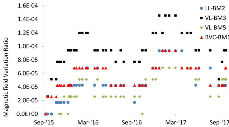
Fig 7 HEBT bending magnet magnetic field variation ratio C350MeV/u
