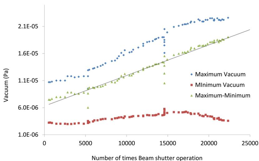
Fig. 9 Vacuum gauge value near the beam shutter and number of beam shutter operations
