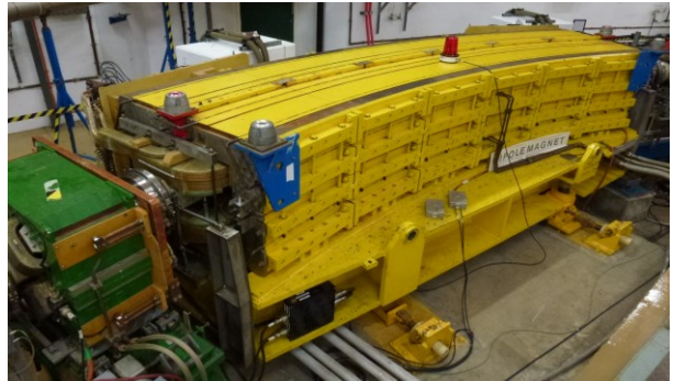
Figure 2 – Synchrotron dipole magnet
