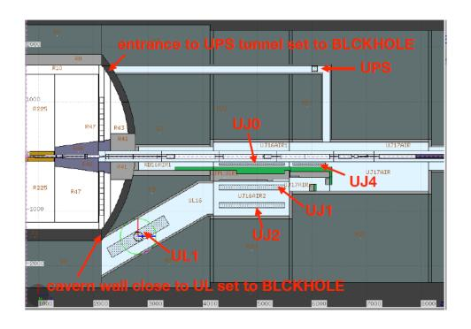
Leakage from UX to UL and UPS not considered in simulation
