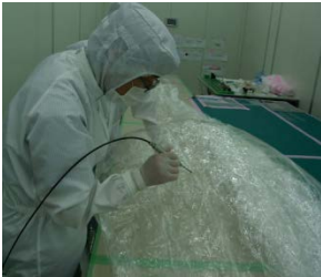
He leak test & Repair work
