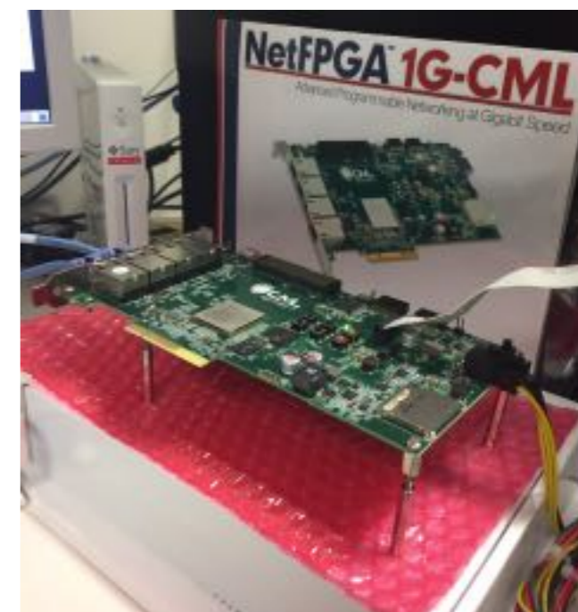
Test Board (FPGA Kintex-7)
